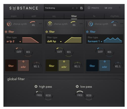
Similar to the EQ Page, the Filter Page allows you to view and edit the settings for each layer at once. Click on the 'filter' and 'adsr' buttons to toggle between settings for the filter envelope and the cutoff/resonance settings. To display SUBSTANCE's filter modes, click on the 'filter type' dropdown box.
